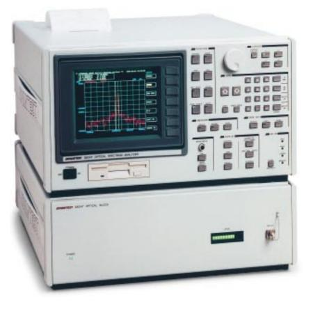
tion can be used. It directly shows the electroluminescence characteristic by fitting a Gaussian distribution into the emission spectrum – a valuable aid in the measurement of erbium-doped fiber amplifiers (EDFA), LDs and Soliton transmission systems.
